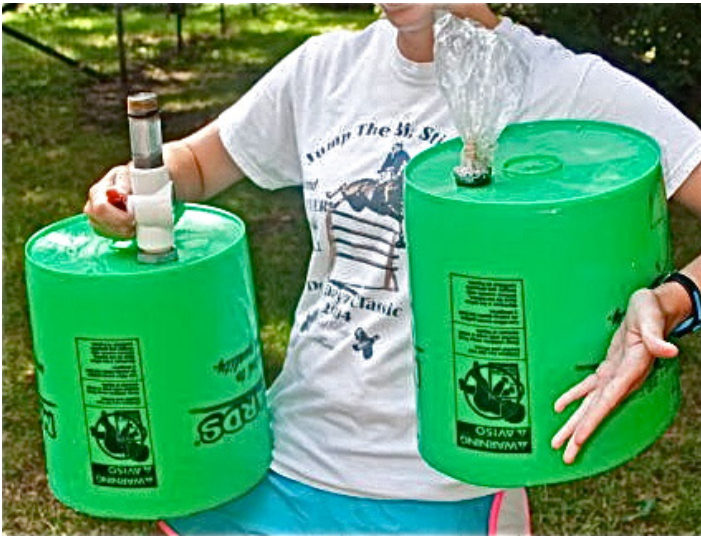
Figure 1. Photograph example of seepage meters used in the field to measure groundwater inflow and groundwater outflow.
