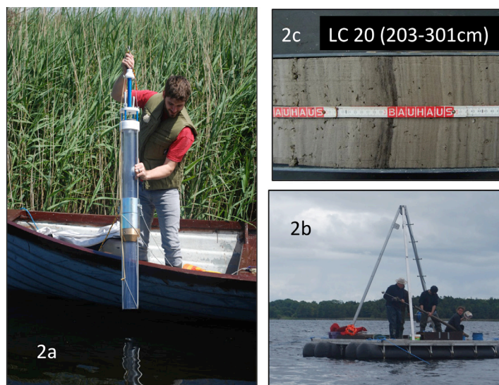
Figure 2: a) Gravity core sampling on Lough Carra, b) Large Usinger piston coring platform, and c) Laminated sediments from core LC 20.
