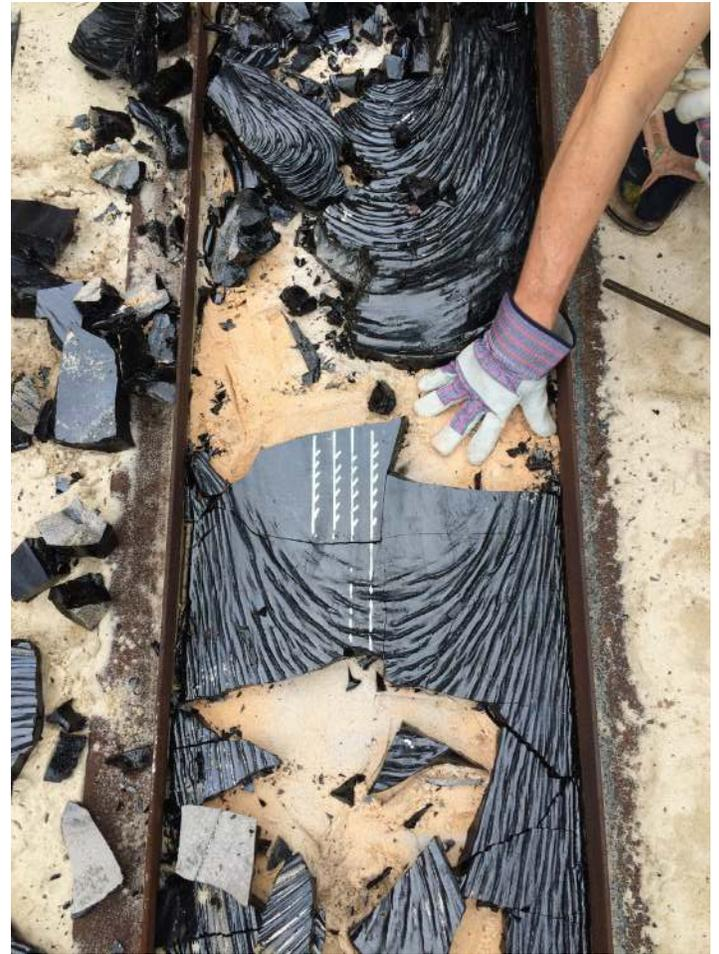
Figure 2. Channelized experimental flow from Syracuse University, New York. Both the core and margins were sampled.
