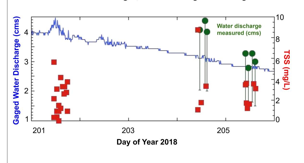
**Fig. 14 (left).** Water discharge reported at the USGS gaging station 05014500 (blue line), measured in the field (green dots, showing 50% uncertainty based on our velocity measurements), and TSS (red squares)
