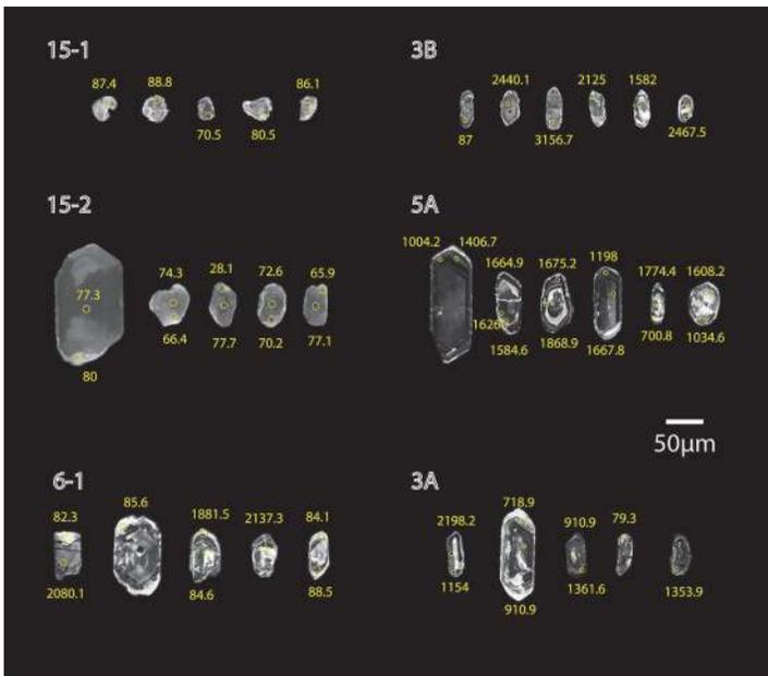
Figure 3. Cathodoluminescence images of zircon separates from a schist and two orthogneisses.
