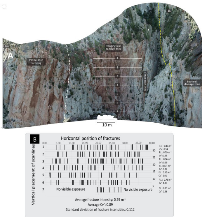
Figure 1. A) Model of the hanging wall with the seven scanlines denoted by thin white lines and labeled with corresponding numbers. The fault is denoted by a yellow dashed line and the boundary of the hanging wall denoted by a dashed white line. B) A graphical representation of the fracture distribution in the hanging wall of the Spencer Bench segment. Fractures are represented by vertical black lines.
