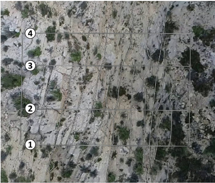
Figure 2. Scanline framework for fracture analysis in the northern section (hanging wall) of the model. Fracture intensity (number of fractures/length of scanline) ranged from \sim 0.20 \text{ m}^{-1} to \sim 0.45 \text{ m}^{-1} .
