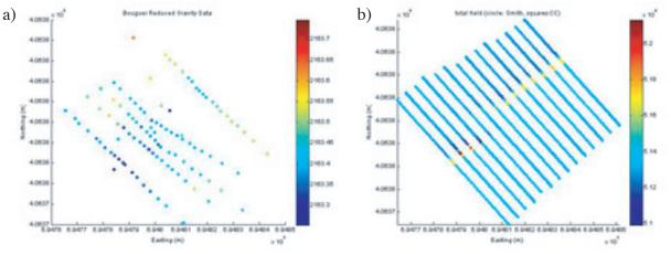
Figure 3. a) Graph of the Bouguer-reduced gravity data.b) Graph of the magnetic data. Both data sets show strong trends along the en echelon dike segments.
