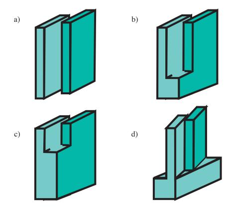
Figure 4. a) The dike segments are not connected. b) The dike segments are connected in the deep subsurface, c) The dike segments are connected in the shallow subsurface, d) The dike segments are rotated with respect to the main dike.
