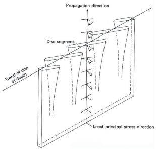
Figure 1. Diagram of the proposed subsurface structure of the northeast dike at Ship Rock, NM (Delaney and Pollard, 1981).
