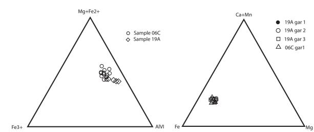
Figure 2: Ternary diagram showing omphacite compositions and Fe2+/Fe3+ zoning over single grains.
