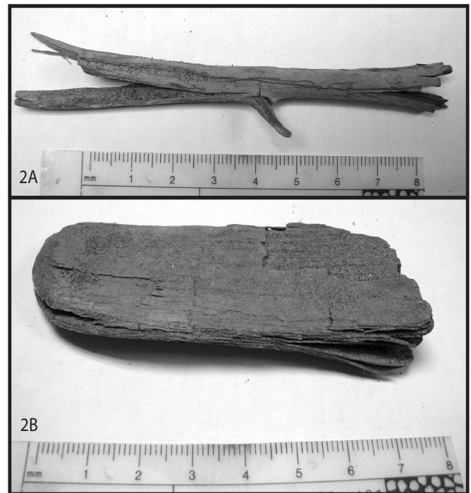
Figure 2. Examples of unworn and worn wood quality. 2A: Unworn wood sample. 2B: Worn wood sample.
