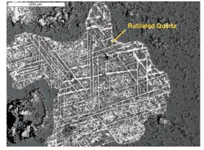
Figure 3. SEM image showing rutilated quartz from sample 27-2.4. Image taken at a working distance of 15mm, an accelerating voltage of 20kv, and a magnification of 180x.
