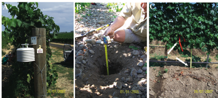
Fig 3. A freestanding HOB0 ambient temperature monitor at Seven Hills vineyard. B Digging pits to bury subsurface HOB0s in Armada vineyard (special thanks to Dr. Pogue). C In situ cluster HOB0 (top arrow) and surface HOB0 (bottom arrow) at Cockburn Hills vineyard.
