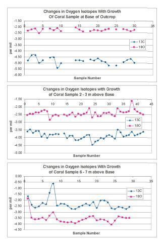
Figure 1. Stable isotope data for 100 cm samples; each sample was drilled at ~1000  $\mu$ m intervals.
