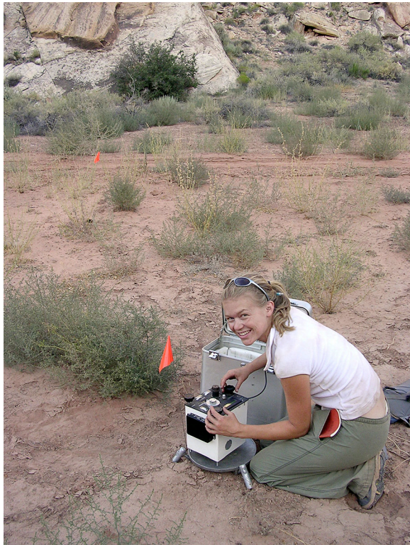
Figure 2. Alice Waldron collecting gravity data using the Lacoste & Romberg Model G meter with Aliod 100 nulling system.
