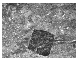
Figure 4: Sample LFL-03-65 (in plane light). This pseudomorph of Hematite after Pyrite postdates the main fabric. The pre-Pyrite growth metamorphic fabric of Glaucophane can be seen running E-W on either side of the crystal.
