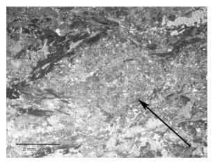
Figure 3: Sample LFL-03-65 (plane light). The approximate mode of the rock is 40% Quartz, 18% Calcite, 15% Phengite, 8% Hematite, 5% Glaucophane, 5% Graphite, 5% Titanite. This rock preserves a pseudomorph after Lawsonite with a boundary preserved by Glaucophane with C-axes
