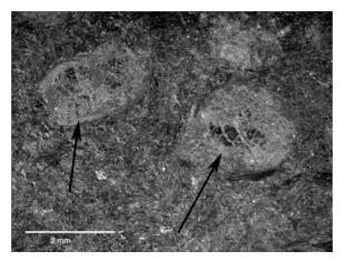
Figure 2: Sample LFL-03-53 (plane light). The approximate mode of the rock is 21% Phengite, 20% Glaucophane, 15% Chlorite, 13% Garnet, 10% Quartz, 7% Graphite, 7% Titanite, 5% Hornblende, 2% Rutile. Garnets (shown) are ~2 mm in diameter and rimmed by retrograde chlorite. A few Garnets in this sample are completely replaced by Chlorite.
