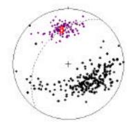
Figure 1: Equal area projection, Bear Creek, CO. S=(216, 45) n=231; L=(35, 350) n=96
