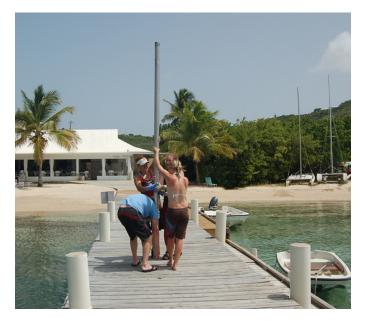
Figure 1. Moving the core from the boat to the core lab on shore required keeping the core vertical to avoid damaging the stratigraphy, especially toward the top of the core.
