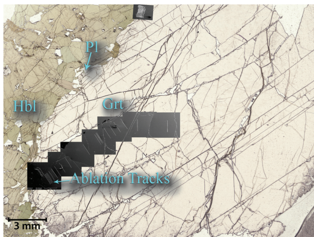
Figure 2. SEM backscatter composite image of ICP-MS analysis tracks overlaid on a plane-polarized thin section image of GM-32-6C. Note the two regions analyzed were combined to create a full profile. For the purposes of this study this garnet was considered concentrically homogenous, which allowed the two transects to be combined. The main set of ablation tracks do not run perpendicular to the garnet rim, and may cut across growth zoning regions.
