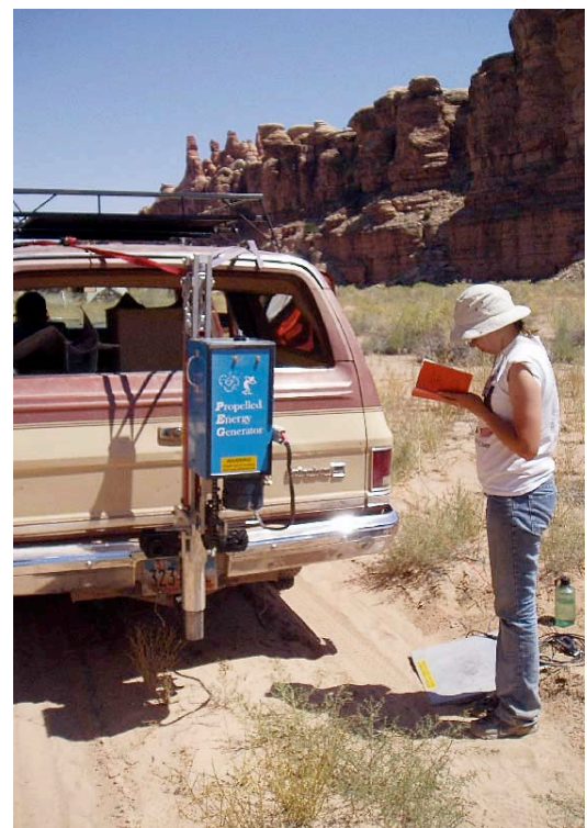
Figure 3. The PEG40 is an advanced accelerated weight drop that weighs 38 kg. It is attached to the back of a truck and powered by a 12-volt battery.
