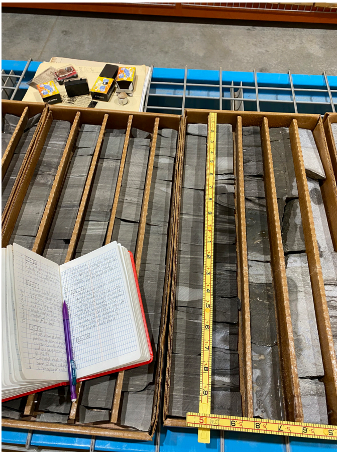
Figure 2. An engineering ruler was used to measure the dimensions of fossils and fossil beds. In addition, changes in sediment color were described as well as the size and location of features, such as pyrite and concretions.
