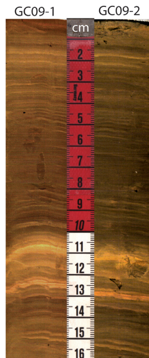
Figure 3. A comparison of two cores taken from Site G. Matching lamination stratigraphy strongly suggests that the top of GC09-2 represents the true sediment-water interface.
