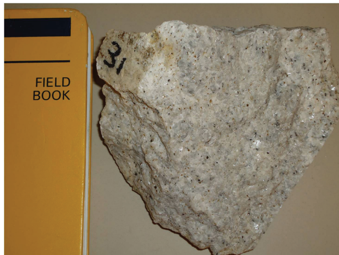
Fig.3. This sample (11BM31) is a typical hand sample of marble collected. Note the white calcite and presence of graphite and silicates. Weathered rinds were removed and not analyzed. Field notebook for scale.
