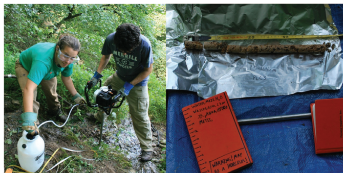
Figure 4: Drilling of tufa (Left) and tufa core being described (Right).
