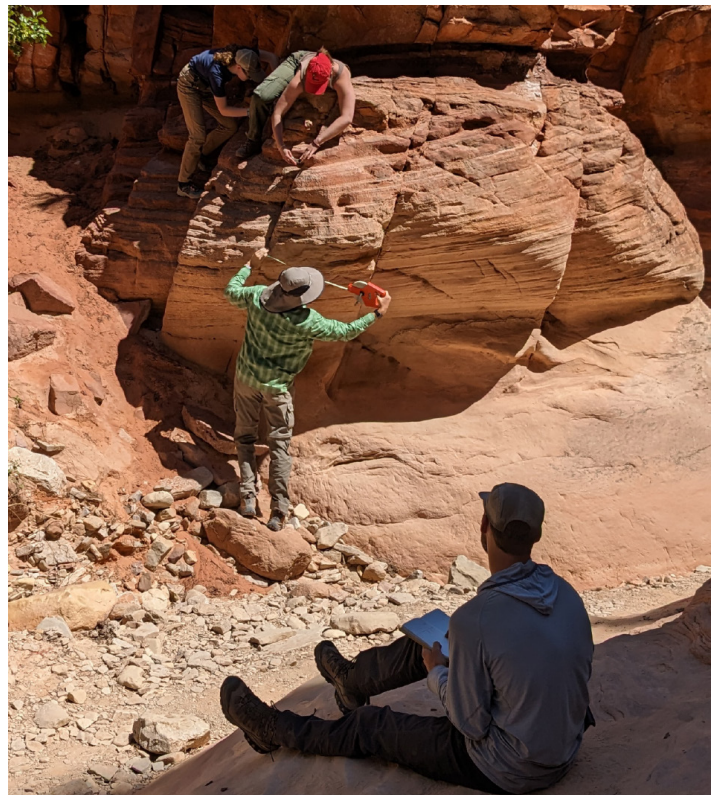
Figure 2. Geologists measuring the attitude of and spacing between fractures along a scanline in Lower Sand Wash.
