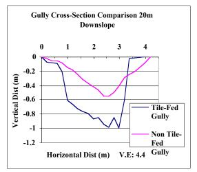
**Figure 2** Comparison of tiled gully and non-tiled gully cross-sections at 20m down slope.
