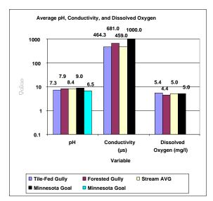
**Figure 4** Average pH, conductivity, and dissolved oxygen levels for the tiled gully, forested gully, and stream.
