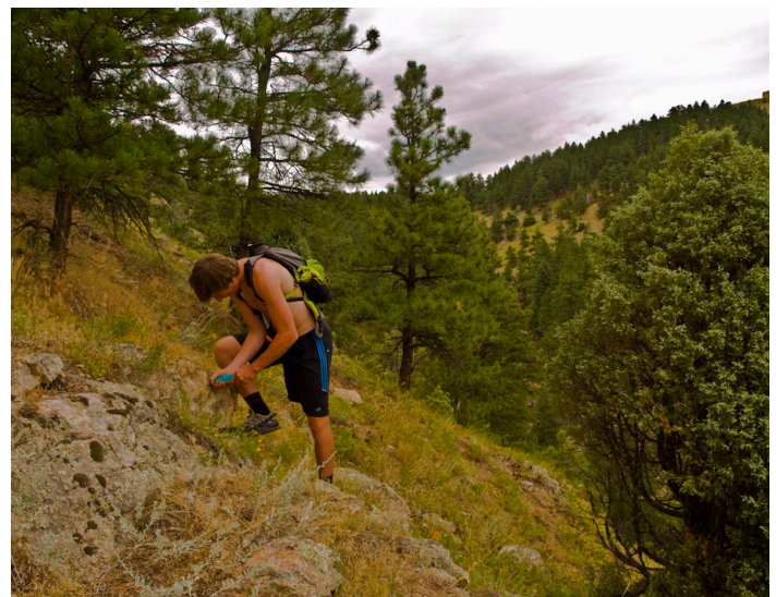
Figure 2. Schmidt hammer measurements being taken on Betasso Gulch hillslopes.
