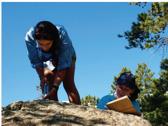
Figure 6. Alex Horne uses Schmidt hammer to collect measurements of compressive strength from weathered gneissic rocks, Gordon Gulch. Sarah Beganskas records values.
