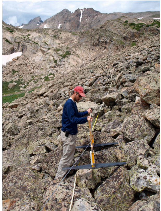
Figure 7. Evan Riddle using ground-penetrating radar on a talus cone, Green Lakes Valley area.
