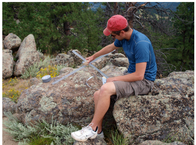
Figure 8. Evan Riddle demonstrates use of block-rounding gauge to estimate the amount of material removed by weathering, Bummars Rock area.
