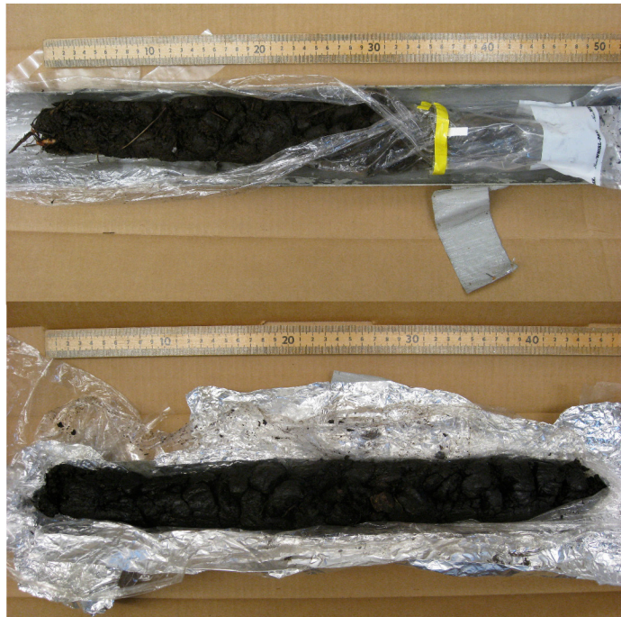
Figure 2: Photos of top two sections of the core. Top photo represents the first meter of core, compacted to 48cm. Bottom picture represents the second meter of core, compacted to 46cm.
