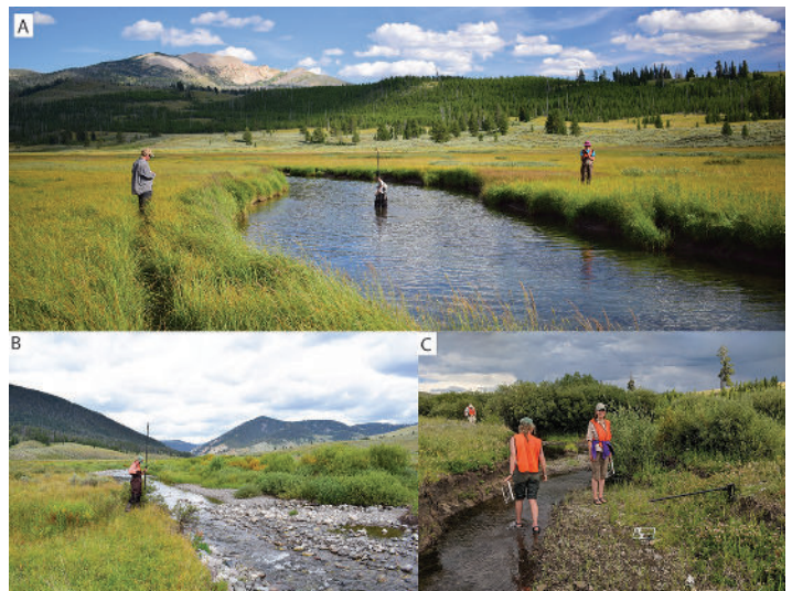
Figure 4. The 2019 Keck Yellowstone Research team surveyed channel geometry using RTK GPS and a total station. The upper reaches of the Gallatin River (A) are relatively low gradient because of local base level control set by recessional moraines (Fig. 3A). Overbank flooding occurs with higher frequency relative to the lower reaches where the river has incised into late Pleistocene outwash deposits (B). The research team characterized bed material using gravelometers and zig-zag pebble counts. Blacktail Deer Creek (C) aggraded during the early and middle Holocene and incised during the late Holocene prior to the historical period.
