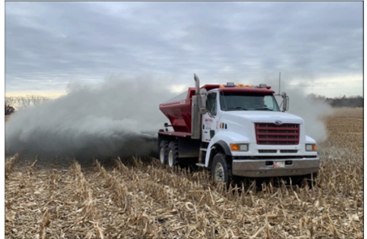
Figure 1. Example of crushed basalt being applied to croplands in this study using spreading equipment designed for lime.
