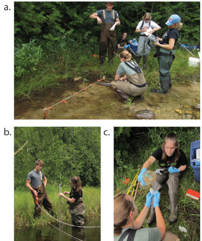
Figure 3. Students worked as a team to (a.) measure geochemical properties along a transect within a sampling array, (b.) measure spring discharge using a wading rod and flow meter, and (c.) sample groundwater after field-filtering.
