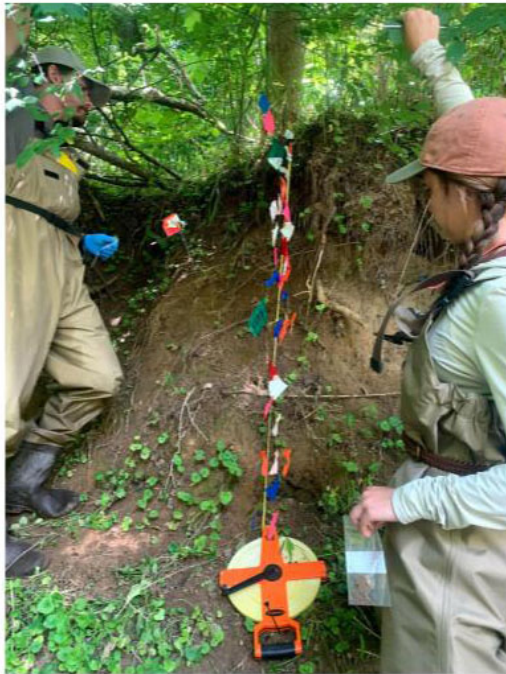
Figure 3. A photo of one of the stratigraphic columns studied by our team. We sampled starting at the top using the tape measure, flags for marking, and lab spatulas to collect the sample. The same method was used at KDPH.
