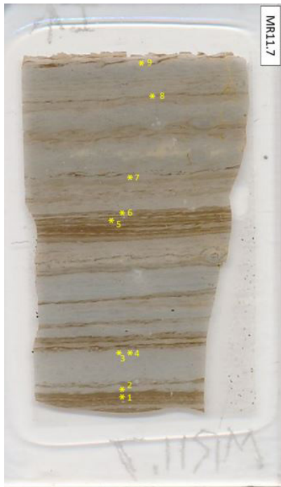
Figure 2. Scan of thin-section MR11.7, showing microlite measurement sites (asterisks) for colorless and brown-colored flow bands along a vertical transect parallel to the stratigraphic “up” position of the oriented rock sample.
