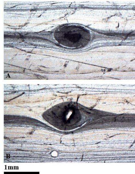
Figure 4. Photomicrographs showing deformation of flow bands around micro-phenocrysts, consistent with simple shear (from sample MR11.9).
