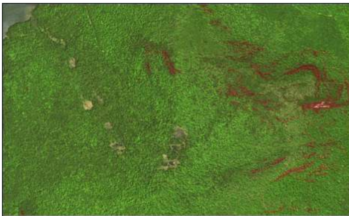
Figure 4. Model of slope throughout the Panther Brook watershed at 10-meter DEM resolution. Areas coded green represent a hillslope angle of less than 30 degrees, areas coded red represent hillslope angles greater than 30 degrees. Dimensions: 1800 m (height) by 3000 m (width).
