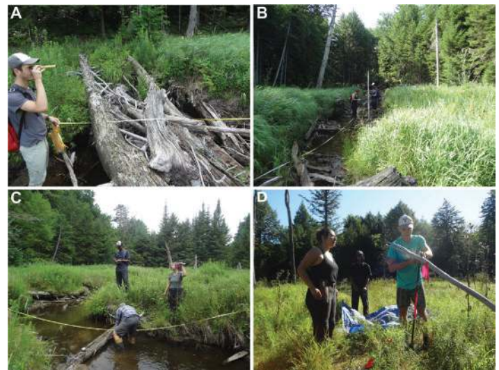
Figure 3. A summary of our field techniques for characterizing the fluvial geomorphology and sediment storage of Panther Brook. (A) Spencer O'Bryan looks 10 m upstream to a survey station occupied by Shyam Das-Toke and Sarah Granke. (B) Shyam holds the stadia rod while Sarah records survey notes. Take note that Panther Brook is incised into beaver meadow sediments through this lowest elevation beaver meadow. (C) Spencer measures LWD while Sarah augers beaver meadow sediment; Shyam records field data. (D) Spencer laboring at the bucket auger while Sarah and Shyam await their turn. Everyone alternated roles between augering, describing sediment textures and colors, and bagging samples.
