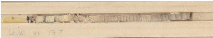
Figure 2. Due to breakage in the core of this white pine, likely the result of rot, the annual ring growth could not be determined. This core, and others like it, are not included in the data set.
