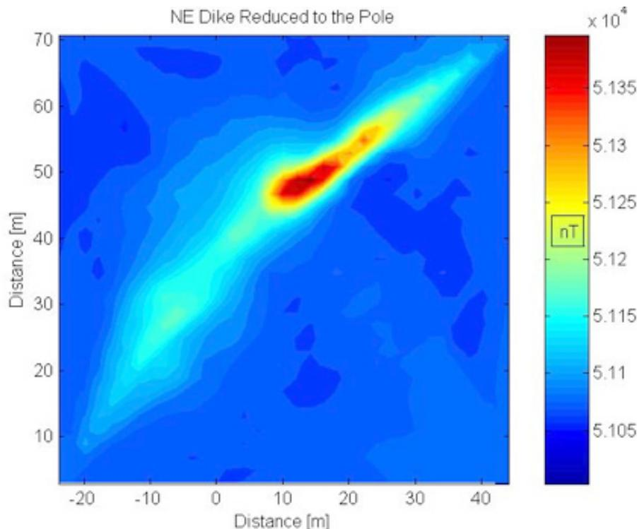
**Fig. 2.** Contoured total field values from the northeast grid rotated in the geomagnetic field and reduced to the pole. Note the irregular intensity of the dike anomaly and the skewness to the northwest. The broadness and heightened intensity in the northern portion of the grid may indicate dike shallowing and thickening. The skewness to the northwest may indicate a northwest dip of the dike. Dike disappears at both ends due to rotation of grid.
