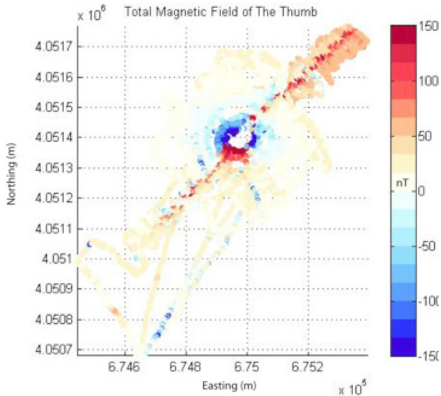
**Fig. 1. Total field magnetic map of The Thumb compiled from ~18,000 magnetometer data and GPS position points in UTM 13 coordinates in Northwest New Mexico. Note presence of The Thumb near the center of the map and the NE-SW trending linear anomaly. No data points were taken atop The Thumb.**
