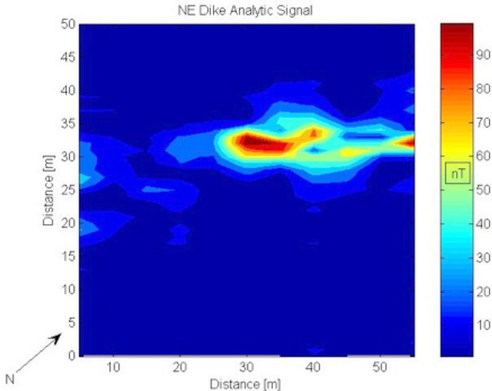
**Fig. 4.** Contoured analytic signal for total field values from the northeast grid (not rotated). Maxima diverge at  $\sim x=35$  m and converge at  $\sim x=50$ m. This observation may represent thickening of the buried body. This observation may also represent an echelon segmentation of the buried body, which is consistent with the segmentation of the NE dike of Ship Rock (Delaney & Pollard, 1981).
