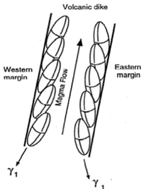
Figure 2. During magma flow, magnetic grains become imbricated along chilled margins. Anisotropy of magnetic susceptibility measures three axes of susceptibility ( $K1$ ,  $K2$ ,  $K3$ ) to determine flow direction. The longest susceptibility axis ( $K1$ ) represents the principle magma flow direction. The shortest susceptibility axis is positioned perpendicular with respect to the long axis (from Tauxe et al., 1998).
