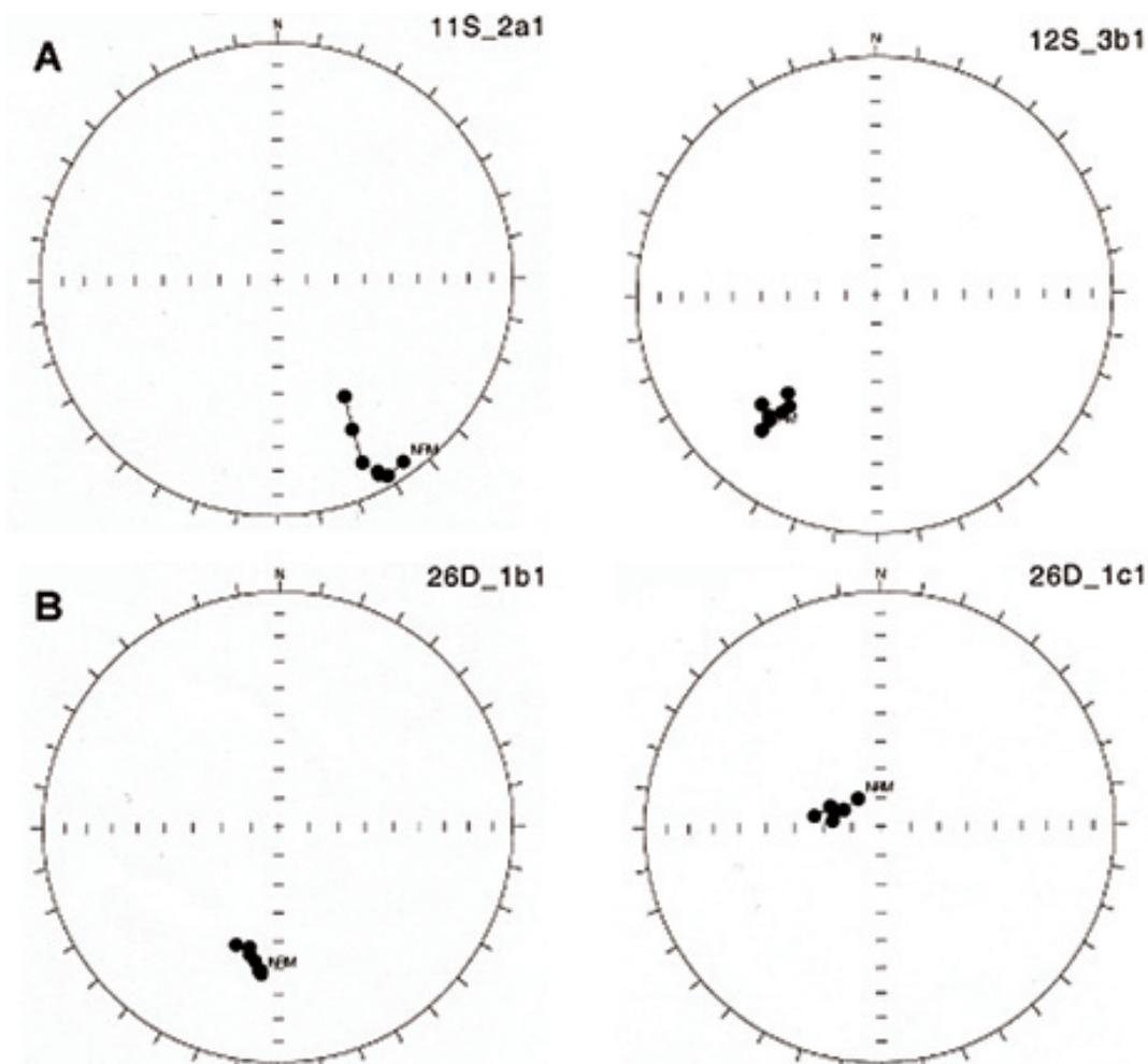
**Figure 5. Natural remanent magnetization for select samples from the Ship Rock radial dike swarm. Ship Rock has a magnetic inclination of 62 degrees, but NRM results show significant variance from this value. A) Samples collected from the south dike display remanence values that are scattered and thus considered unstable. B) Remanence values taken from diatreme sample show significantly different values further indicating instability**
