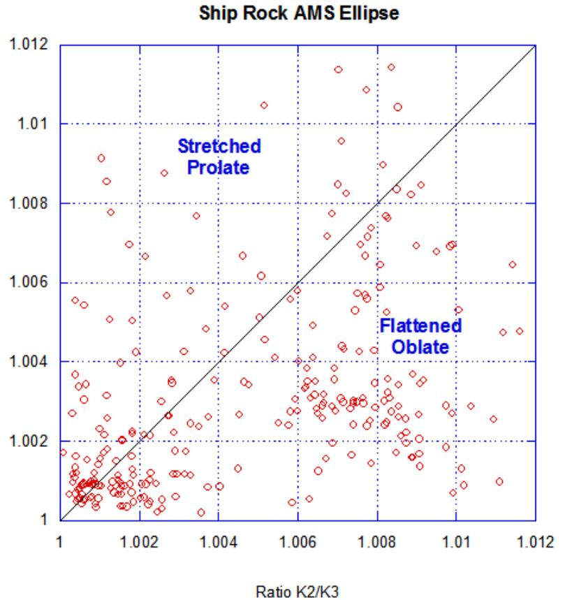
Figure 3. Flinn diagram comparing the ratios of the maximum and intermediate susceptibility values ( $K1/K2$ ) to the intermediate and minimum susceptibility values ( $K2/K3$ ) to determine ellipse shape of Ship Rock samples analyzed by AMS. The graph points show some scatter, but clustering indicates oblate and spherical ellipse shape.
