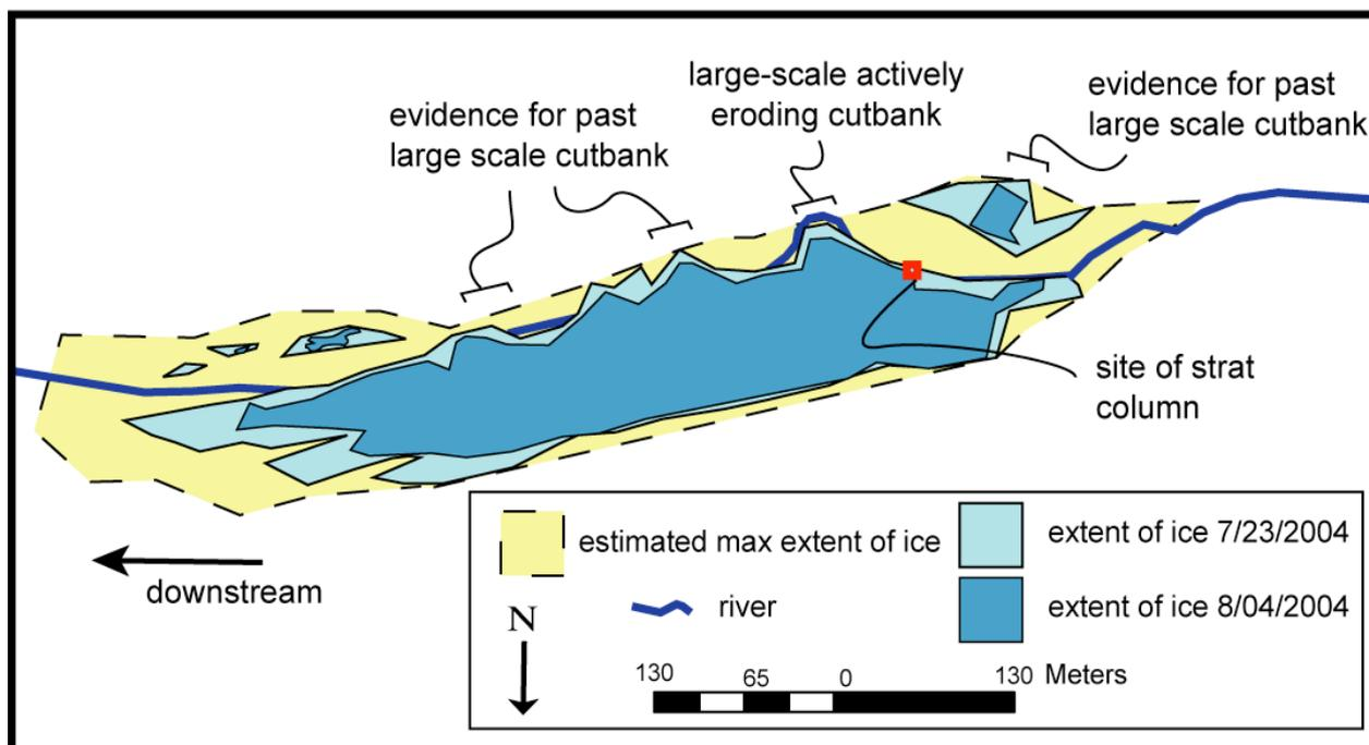
**Figure 1.** Map of aufeis sheet made with GPS measurements taken at the beginning of student (7/23/2004) and the end (8/04/2004). Features such as the stream, major cutbanks and the location of the stratigraphic column (see Fig. 2) were also mapped with a GPS.
