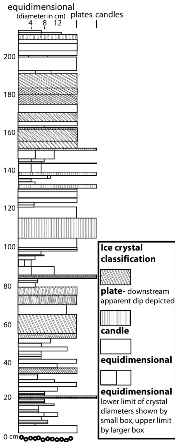
Figure 2. Stratigraphic column for a 2.15-m section of the aufeis sheet comprised of 90 laminations. Ice crystals are grouped into three morphologies: equidimensional, candle, and plate. Often the plates of ice align so they dip downstream. Where this is measured, the dip angle of the plate is shown except where there was no recognized preferential orientation.
