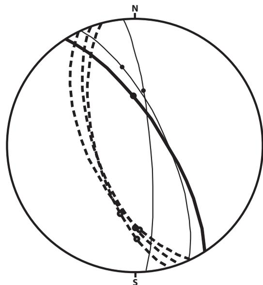
**Figure 3:** Equal-area stereonet of groove rakes (dots) and related fault planes at Diapori (dashed), Katakefalos (bold), and Charasonas (fine). Groove axes occur parallel to the direction of displacement. Grooves in west-dipping planes at Diapori show oblique slip to the south, while grooves in east-dipping planes at Katakefalos and Charasonas show oblique slip to the north.
