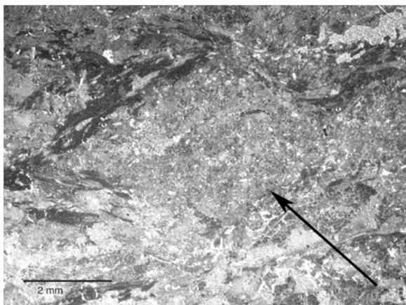
**Figure 3: Sample LFL-03-65 (plane light). The approximate mode of the rock is 40% Quartz, 18% Calcite, 15% Phengite, 8% Hematite, 5% Glauco-phane, 5% Graphite, 5% Titanite. This rock preserves a pseudomorph after Lawsonite with a boundary preserved by Glauco-phane with C-axes**
