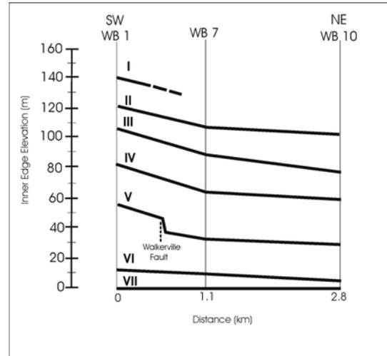
**Figure 3: Terrace inner edge elevations plotted in a line perpendicular to profiles WB 1, 7 and 10.**
