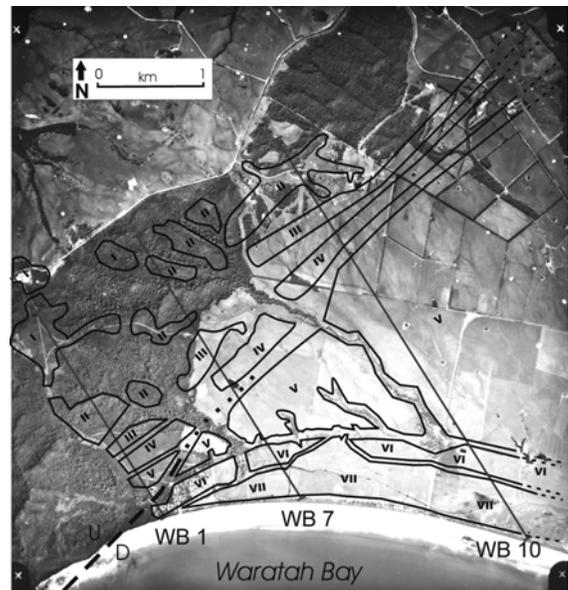
**Figure 1: Marine terrace treads of Waratah Bay mapped on an aerial photo base. Gray lines mark locations of projected terrace profiles WB 1, 7, and 10 (Fig. 2).**
