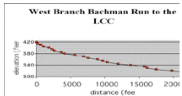
Figure 2 Longitudinal profile for the West Branch Bachman Run deviates from an expected exponential curve.
