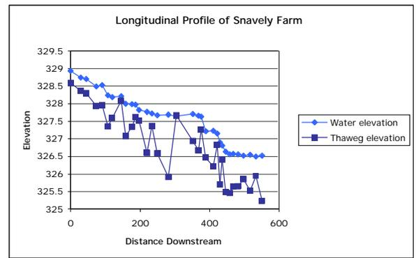
**Fig. 3. Longitudinal profile of Snavely farm, showing the more healthy, tighter pool-riffle system.**
