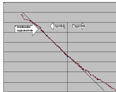
**Fig 4. Longitudinal Profile of Millers Run, Showing the Areas of aggradation and degradation.**
