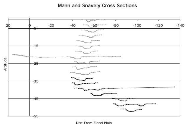
**Fig 1. Cross sections of the Mann and Snavelly Farms, showing the change from v-shaped profiles to less healthy, u-shaped profiles.**
