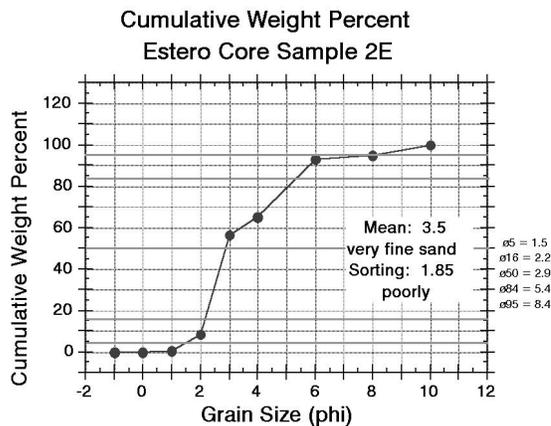
**Fig. 2.** Chart showing cumulative weight percent and grain size distribution from near the top of Core 2, Facies E, as determined from coarse-grain sieve and fine-grain pipette sedimentary analyses.
