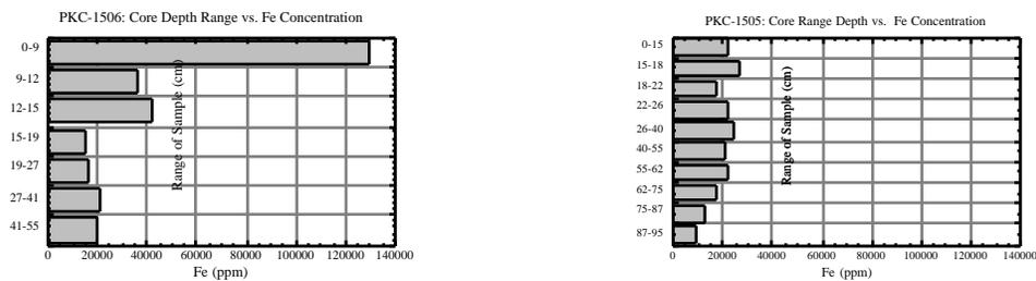
**Figure 2:** Plots showing both temporal and spatial distribution of Fe. PKC-1506 shows a decrease in metal concentration as core depth increases. Comparison of the two plots shows that PKC-1506, which was taken by the main seep has much higher metal concentration than PKC-1505, which was taken on the side of the wetland farthest from the seep.
