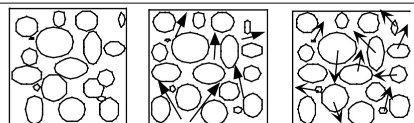
**Figure 1.** a) Sediment grains loosely packed, water in interstitial pore spaces. b) Increase in pore-water pressure, water begins to move "floating" grains. c) Grains themselves move, mixture flows.
