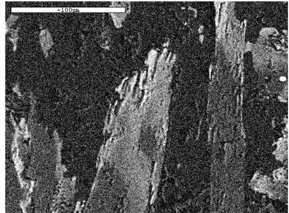
Figure 2. Backscattered electron image of zoned glaucophane.
