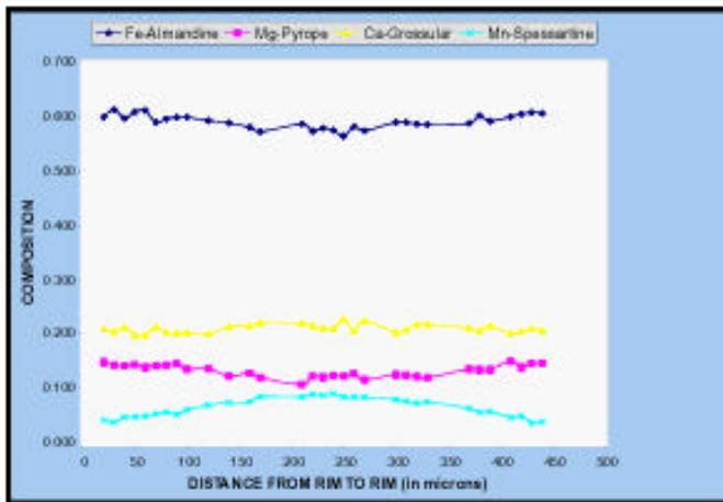
FIGURE 7 : Garnet traverse, from an Fe-Ti metagabbro, showing grossular-spessartine-almandine-pyrope compositions
