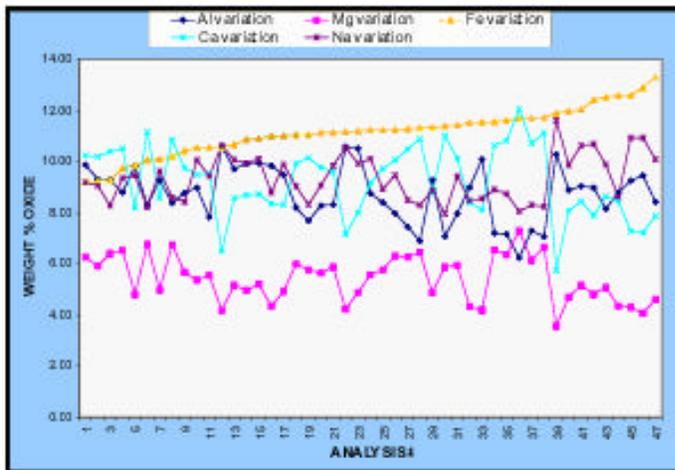
FIGURE 5 : Clinopyroxene Chemical variation according to weight percent distribution of the elements based on multiple analyses on a single slide. The inverse relationship between the diopside and the jadeite component, and the variation in their constituent elements reflect the pressure sensitive diopside-jadeite substitution.
