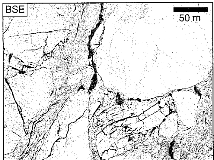
Figure 3. Backscattered electron image of brittle behavior in greywacke gouge. Note the highly fractured grains and lack of a dominant foliation. Material is primarily quartz, potassium feldspar, and clay.
